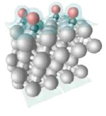
fcc (CO@Pt<sub>3</sub>) E<sub>DFT</sub> = 0 eV V<sub>DFT</sub> = 1743 cm<sup>-1</sup> V<sub>exp</sub> = 1780 cm<sup>-1</sup>
