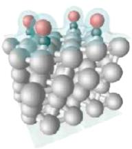
bridge (CO@Pt<sub>2</sub>)  $E_{DFT}$  = +0.03 eV  $V_{DFT}$  = 1845 cm<sup>-1</sup>  $V_{exp}$  = 1830 cm<sup>-1</sup>
