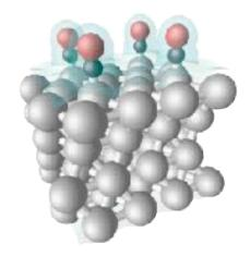
atop (CO@Pt<sub>1</sub>) E<sub>DFT</sub> = +0.10 eV V<sub>DFT</sub> = 2050 cm<sup>-1</sup> V<sub>exp</sub> = 2070 cm<sup>-1</sup>
