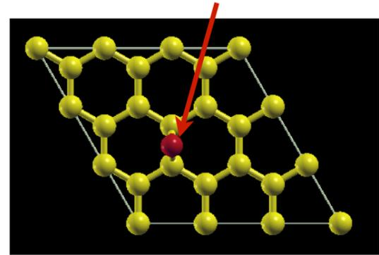
This example consists of two tasks: (i) build a  $(3 \times 3)$  supercell of graphene; (ii) add an O atom onto graphene- $(3 \times 3)$  supercell structure and run a relaxation calculation.
