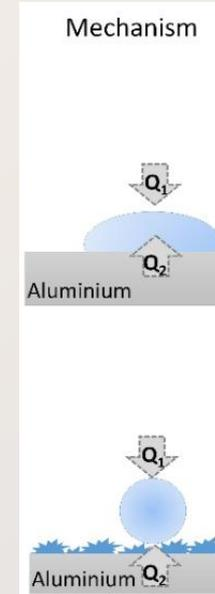
Anti-icing properties of a) ground and b) grafted aluminium with FAS-10. Samples were cooled to  $-20\text{ }^{\circ}\text{C}$ . Water droplet was dropped on the surface.
